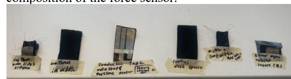
Figure 2. The six iterations of tested force sensors. (For Table 1: Left to Right A, B, C, D, E, F)
